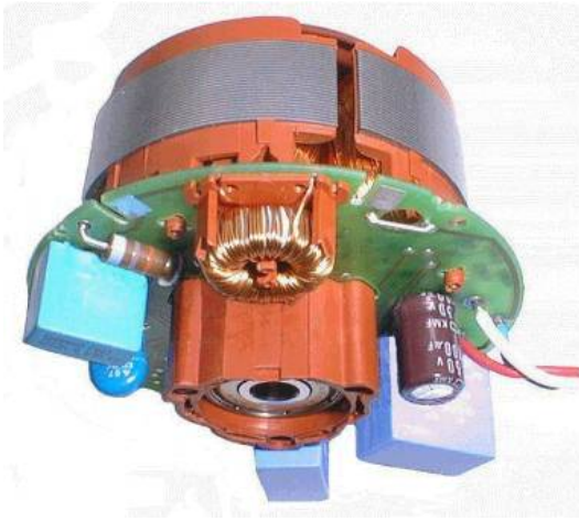
Fig. 7. The starting electronic circuit integrated into the motor flange
